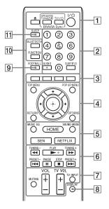
Number 5, AUDIO, VOL +, and buttons have a tactile dot. Use the tactile dot as a reference when operating the remote control.
