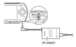
Plug the AC power cord into an electrical outlet.
