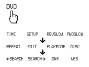
2 Press the desired key in the touch-key display.When the remote control signal is sent, is displayed on the display.
