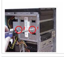
**Step 8.** Using the enclosed magnetic screwdriver, reinstall the previously removed screwsfollowing the above sequence. (In this example: the lower optical drive.) **IMPORTANT!** Do not over tighten the screws!
