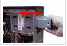
**Step 7.** Carefully slide the new optical drive into the newly vacant space in the chassis, making sure the screw holes are aligned.
