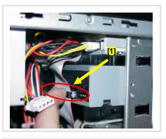
**Step 9.** Reconnect the IDE data cable [1] and the power cable [2] to the new optical disk drive you have replaced. (In this example: the lower optical drive.)
