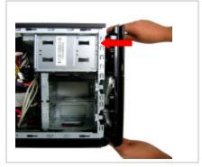
**Step 10.** Reinstall the front panel to its original position, as shown.
