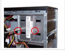
**Step 5.** Using the enclosed magnetic screwdriver, remove the two(2) screw s from the optical drive you are replacing. (In this example the lower optical drive.)
