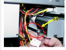
**Step 4.** Remove the power connector [1] and the IDE data cable [2] from the optical disk drive you are replacing. (In this example: the lower optical drive.) **NOTE** Your PC may be equipped with more than one optical disk drive.
