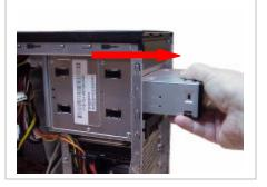
**Step 6.** Pull out the original optical drive from the chassis in the direction of the arrow.
