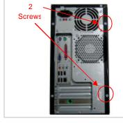
**Step 11.** Reinstall the left chassis cover panel in the direction of arrow Then using the enclosed magnetic screwdriver, reinstall the two (2) previously removed screws. **IMPORTANT!** Do not over tighten the screw s! Return the original optical disk drive to Sony following the included shipping instructions
