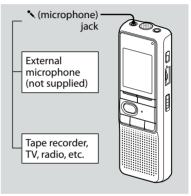
1 Connect a plug-in-power type microphone or other equipment to the \*(microphone) jack. When you connect an external microphone, the built-in microphone is automatically cut off. When a plug in power type microphone is connected, power is automatically supplied to the microphone from the IC recorder.
