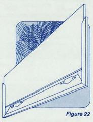
**D)** Reattach the top frame by reinstalling the two top corner screws.
