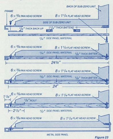
Anchor the side panel with decorative headed screws (as shown) or finishing nails can be used. The screws/ nails must be obtained from your local hardware supply store.
