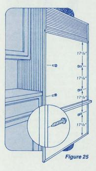
**1)** Drill three (3) <sup>3</sup>/<sub>16</sub>" holes (per specs in Figure 25) through both outer trims.
