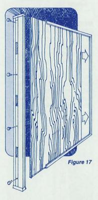
**D)** With panel in position, replace handle and screws. Replace the trim molding(s) by inserting the top and then the bottom into the handle channel. Release the middle and set the magnets.
