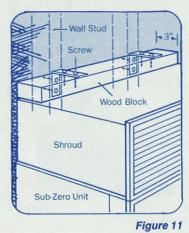
To block the unit, using the wood block and hardware provided, follow these steps.
