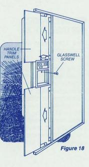
**D)** Next, remove the water and ice glasswell by removing the mounting screw. Then slide the glasswell up and pull out as in Figure 18.
