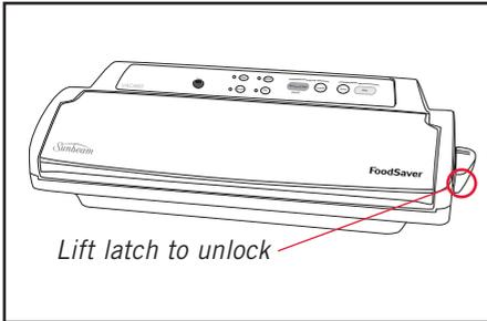
5. Place one open end of the bag material across the sealing strip and close lid. (Do not place edge of bag into vacuum channel when sealing bags)
