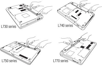
(Sample Illustration) Removing the battery
