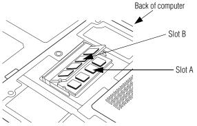
(Sample Illustration) Removing the memory module
