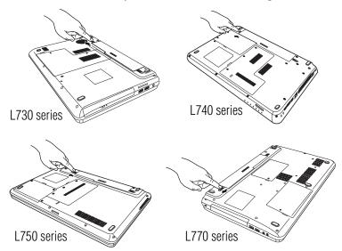
(Sample Illustration) Unlocking the battery release lock
