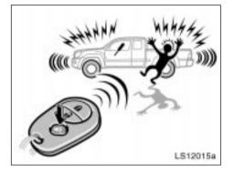
Pushing the "**■** " (alarm) switch blows the horn intermittently and flashes the headlights, tail lights, turn signal lights, and interior light.
