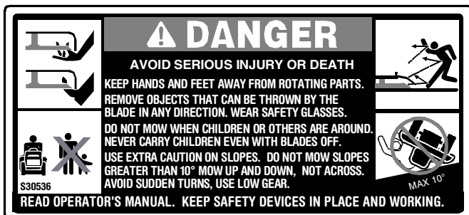
Label shape may vary by tractor model. Label contents do not vary.
