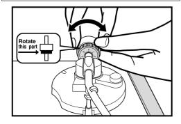
As shown in the illustration, overhang indicates the distance from the stylus tip to the center of the turntable spindle when the stylus tip falls on the extension of a straight line from the pivot of the tonearm to the center of the spindle. If this adjustment is not correct, the stylus will not track the grooves properly.
