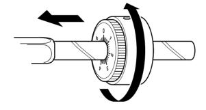
t Slide balanceweight onto rear of tonearm with the number scale facing the cartridge end. Twist lightly to screw into position.
