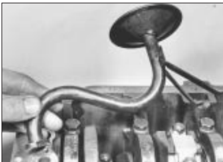
16.3 Removing oil pump pick-up tube and strainer
