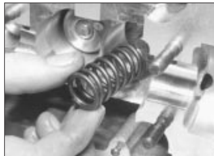
5.11b Removing an inner valve spring
