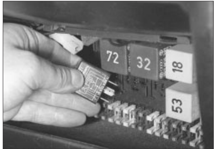
3.3 Removing a relay
