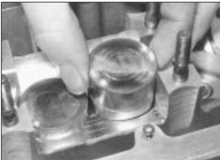
5.4 Removing an hydraulic bucket tappet
