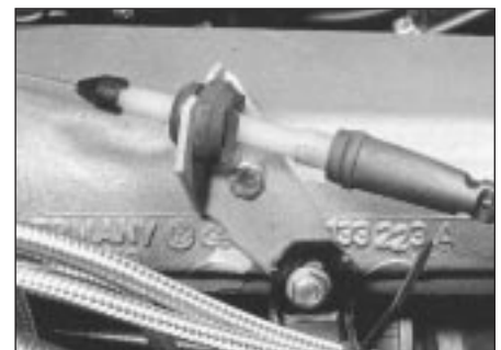
8.10 Accelerator cable adjuster and support bracket
