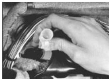
16.4 Disconnect speedometer cable
