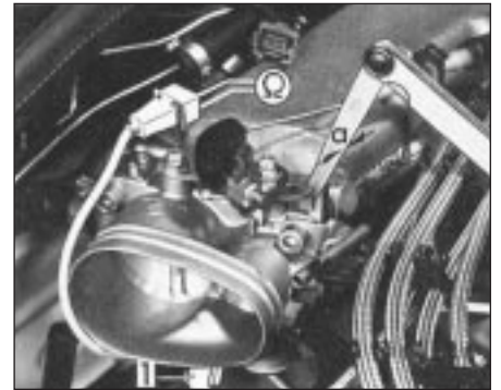
12.10 Throttle valve switch check
