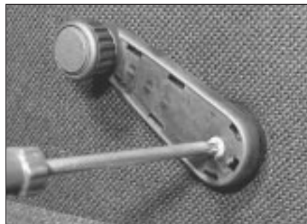
14.4b . . . and handle retaining screw
