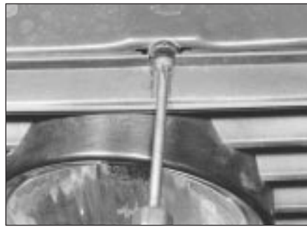
8.2 Undoing front grille retaining screws
