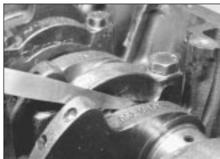
18.3 Checking crankshaft endfloat
