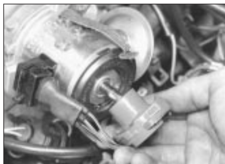
11.9 Fitting rotor arm
