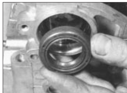
10.15 Removing camshaft oil seal
