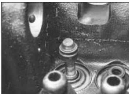
34.4 . . . then fit the new oil seal
