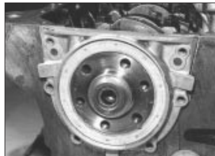
30.9 Fitting crankshaft rear oil seal and flange
