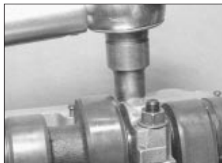
10.5 Tightening a camshaft bearing cap nut
