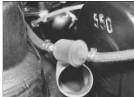
33.1 In-line fuel filter - 1.05 and 1.3 litre, carburettor
