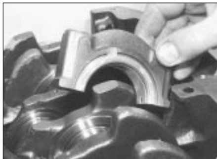
30.5 Fitting main bearing caps
