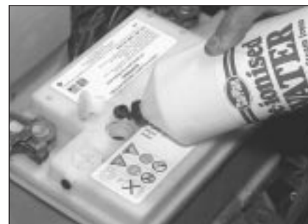
7.3b . . . and top up electrolyte level using distilled or de-ionised water
