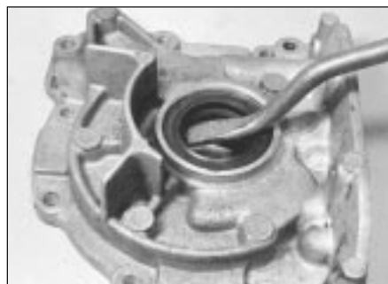
31.1 Prising out oil pump oil seal
