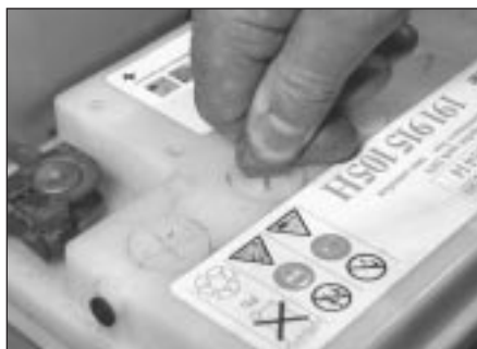
7.3a Remove battery filler caps . . .
