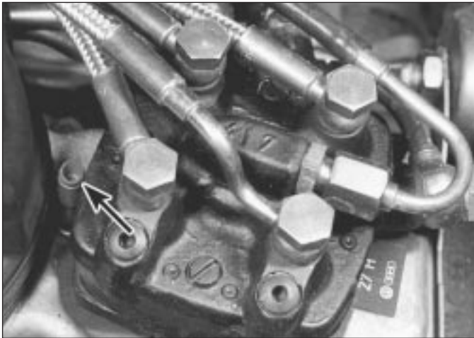
7.2 Idle CO adjustment screw location (arrowed)
