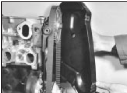
9.4 Removing timing cover
