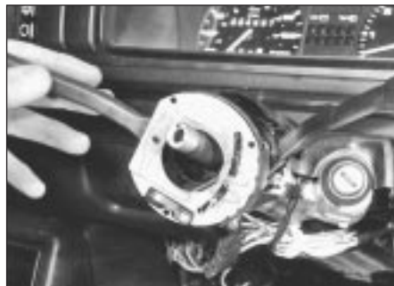
12.6 Removing indicator switch . . .
