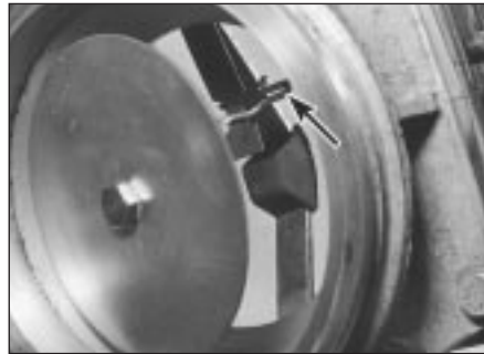
14.6 Airflow sensor plate adjustment clip (arrowed)
