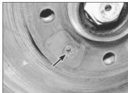
4.5 Front brake disc retaining screw (arrowed)
