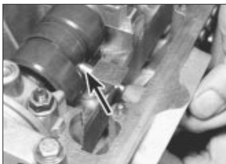
11.6 Fitting fuel pump plunger (arrowed)
