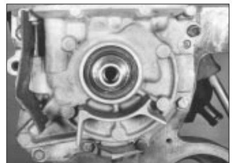
31.4 Fitted location of oil pump
