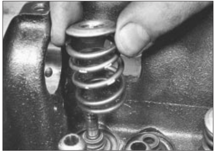
11.2b Removing valve springs and retainers . . .
