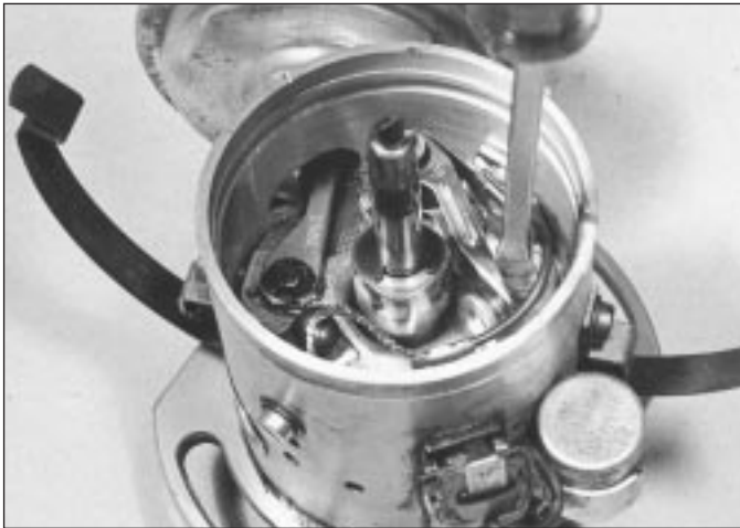
16.10b Adjusting contact breaker points gap
