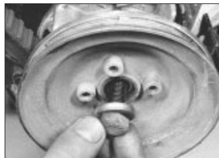
12.7 Removing crankshaft sprocket bolt and washer
