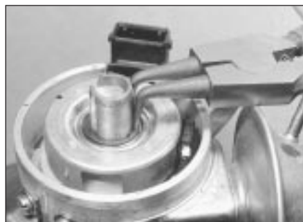
7.4a Remove the locking ring and rotor . . .
