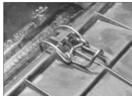
32.4a Unclip air cleaner cover . . .
