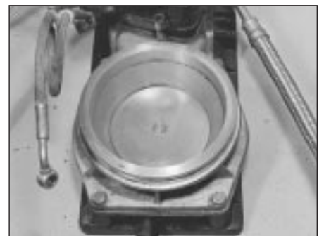
14.2 Top view of airflow sensor plate
