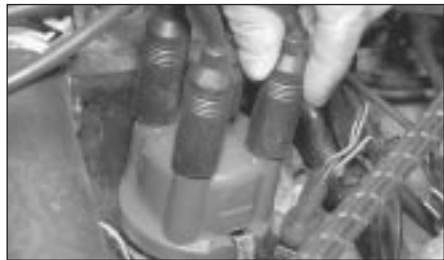
A Check that the HT lead connections at the distributor are clean and make sure they are secure by pushing them onto the cap.
