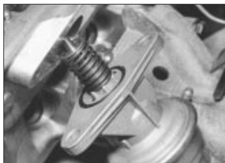
11.7a Fitting fuel pump
