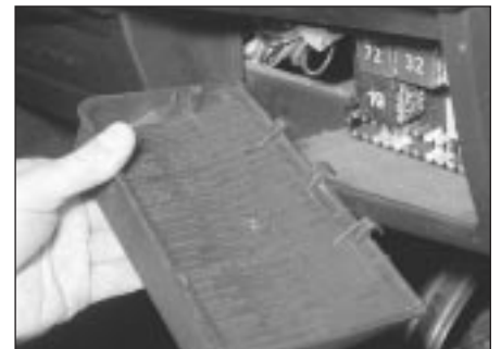
3.1 Removing fuse/relay unit cover
