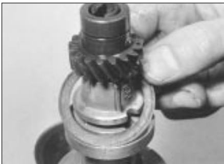
6.6b The gasket must be removed
