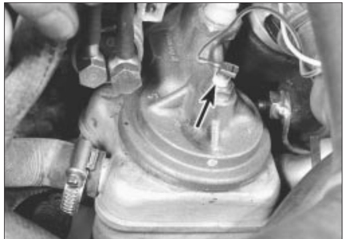
5.39 Oil temperature sender (arrowed)
