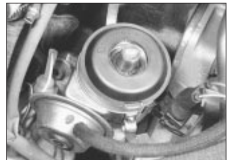
7.3b . . . and lift off the dust cap
