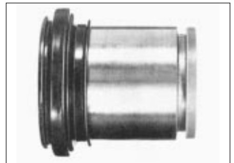
3.9 Dust seal location on caliper piston
