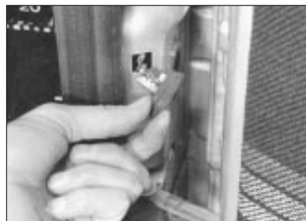
14.3 Door courtesy light switch removal
