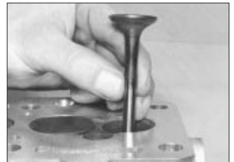
5.12 Removing a valve
