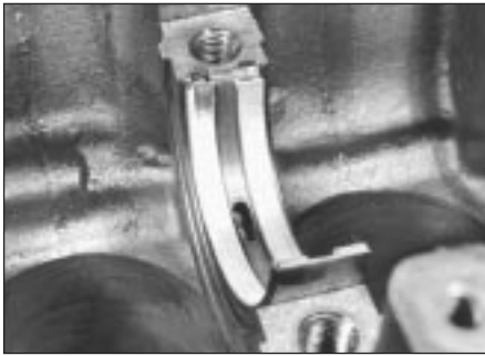
29.2 Fitting centre main bearing shell
