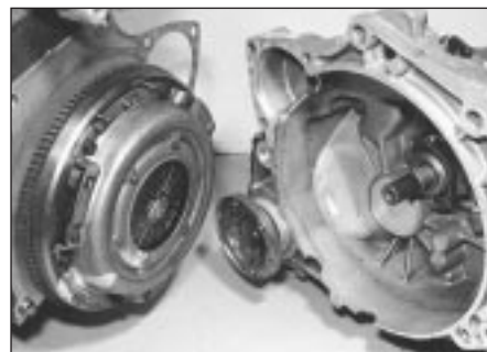
6.6b . . . then separate engine and transmission
