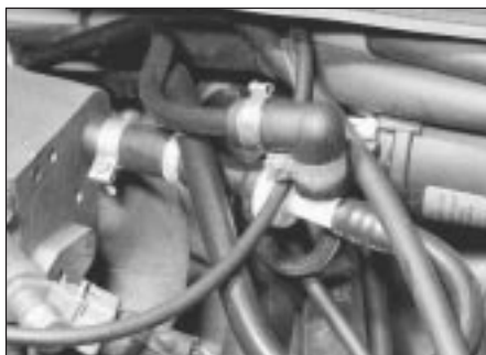
23.5 Vacuum hose-to-cylinder connector
