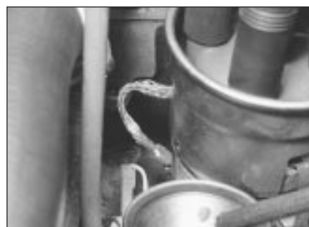
6.2 Transistorised distributor earth lead connection to body (from screen)
