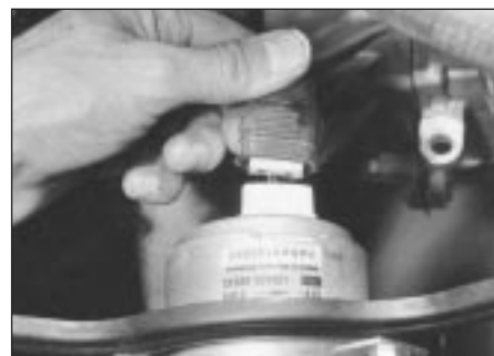
3.3b Detach cooling fan lead connector
