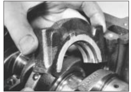
29.4 Fitting centre main bearing cap
