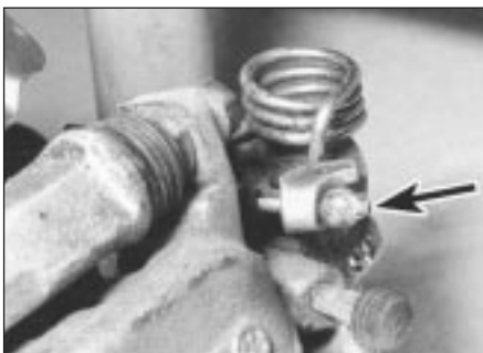
2.15 Release handbrake cable (arrowed) from caliper
