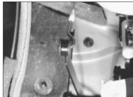
10.5 Accelerator cable-to-pedal attachment
