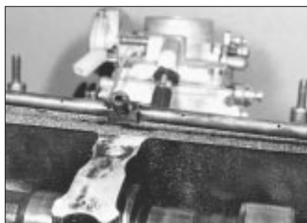
10.7 Removing oil spray tube
