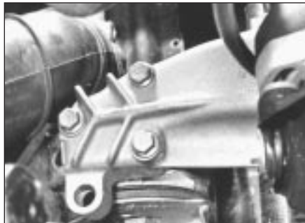
5.24 Engine mounting/bearer - right-hand
