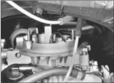
3.3a Disconnecting temperature sensor hose ...
