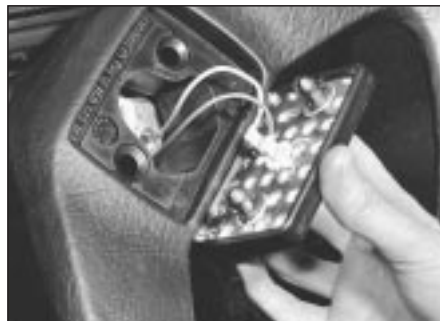
11.3a Removing steering wheel centre cover - 1.3 litre
