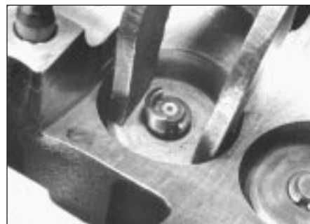
12.12c . . . and valve collets
