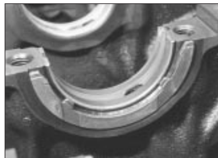
30.3c . . . together with thrustwashers
