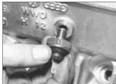
11.3 Refitting oil pressure switch
