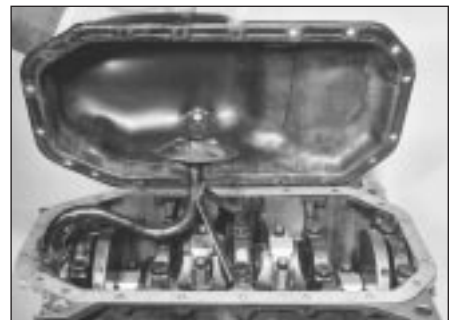
15.2 Removing the sump
