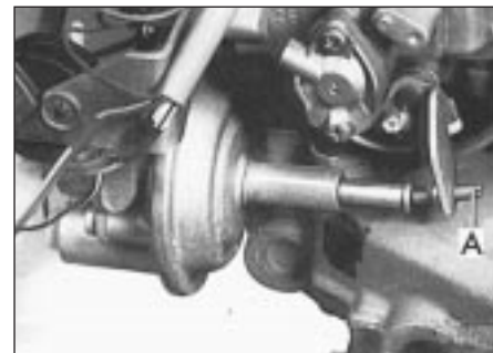
17.39b Fast idle adjustment screw (A)
