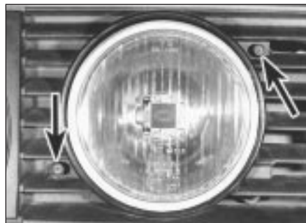
7.4 Foglight beam alignment adjuster screws (arrowed)
