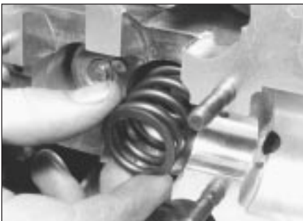
5.11a Removing an outer valve spring
