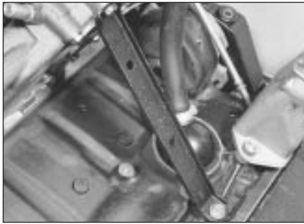
19.5 Inlet manifold support stay - 1.3 litre
