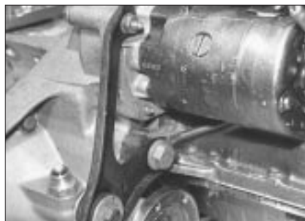
6.3 Starter motor and exhaust support bracket
