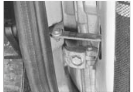
16.1 Door check strap and hinge
