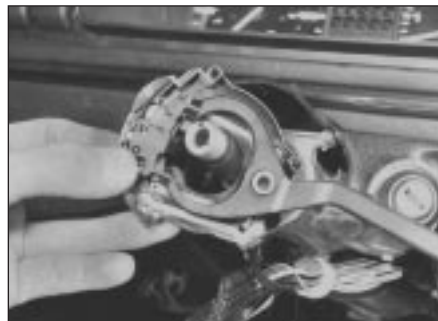
12.7a . . . and wiper control switch
