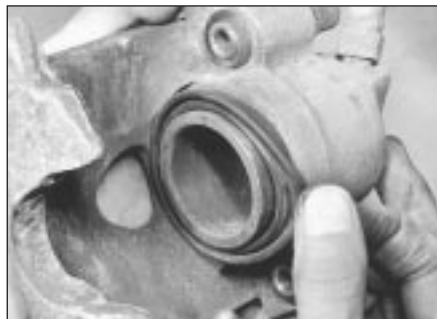
3.5 Removing the dust seal
