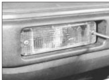
8.4 Front indicator lens removal
