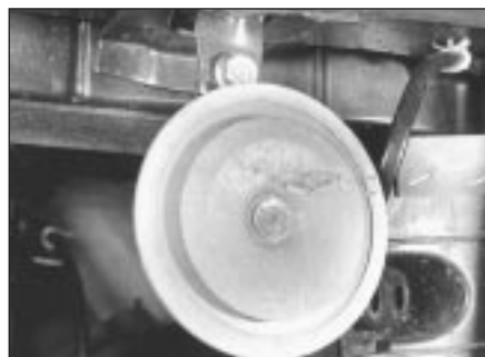
24.1a Single horn location behind front grille
