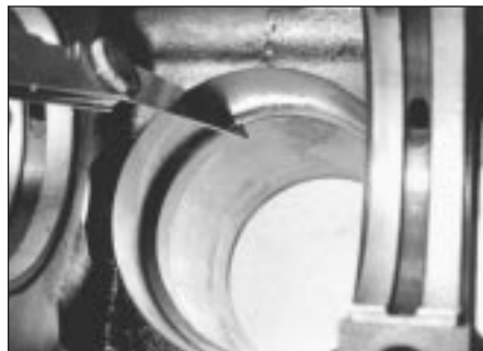
23.6 Checking piston ring gaps
