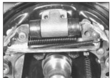
6.11 Wheel cylinder, upper return spring and pushrod assembly
