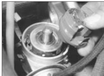
7.3a Pull free the rotor . . .
