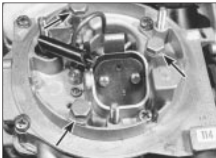
13.8 Carburettor securing bolts (arrowed) - Pierburg/Solex 2E3
