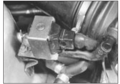
5.2 Increased idling speed valve (air conditioned models)
