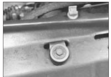
3.5 Radiator central retaining bolt and bracket
