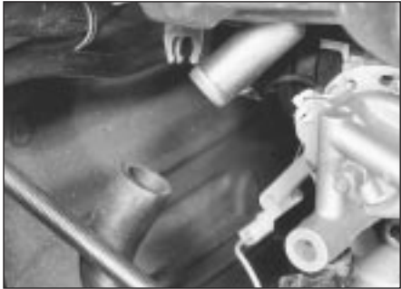
3.3b ... and crankcase emission hose - 1.3 litre
