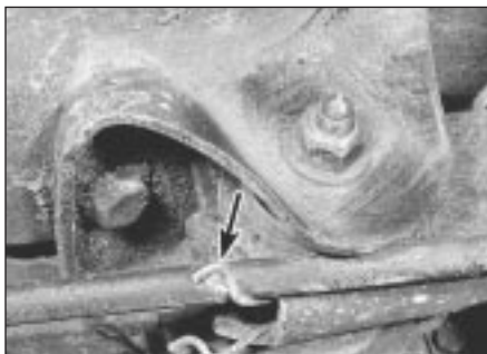
14.6 Handbrake cable retaining clip (arrowed) at rear axle beam pivot
