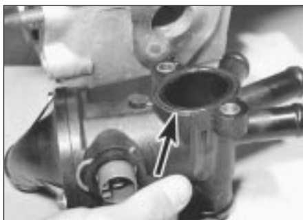
11.4 O-ring (arrowed) in thermostat housing
