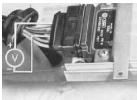
5.4 Voltmeter connection when testing Hall sender
