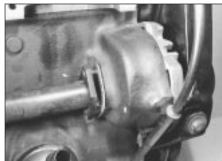
8.1d Removing engine rear coolant pipe
