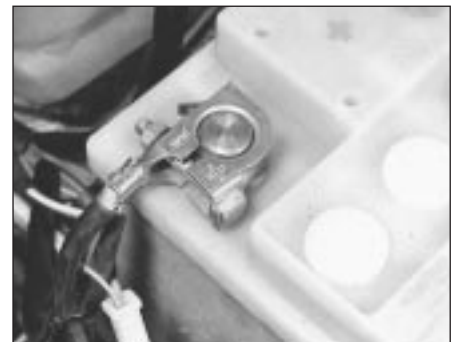
4.2 Battery positive terminal connection
