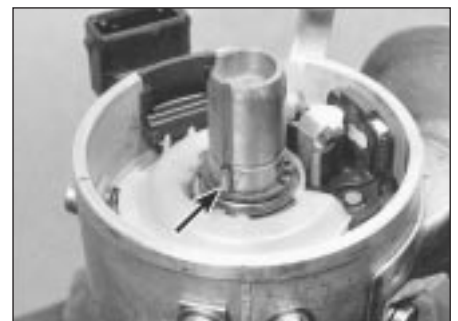
7.4b . . . and locating pin from shaft groove (arrowed)
