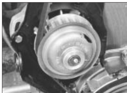
6.5 Disengage timing belt from coolant pump sprocket
