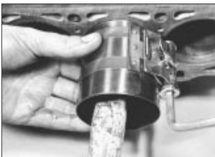
30.4 Using a piston ring compressor
