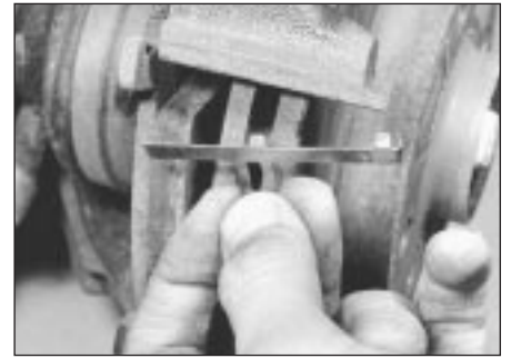
2.5 Removing a pad retaining spring
