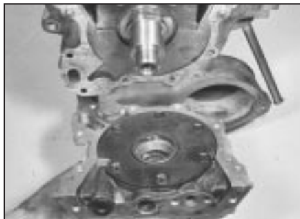
16.4a Removing oil pump . . .
