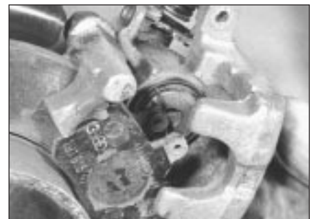
2.17 Rear brake caliper removal
