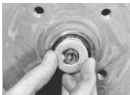
6.5b ... remove the thrustwasher ...
