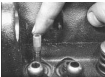
34.3 Locate plastic sleeve on valve stem . . .
