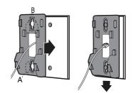
3. Align the grooves on the telephone base with the tabs on the wall mount bracket, and then slide it down until it clicks securely in place.
