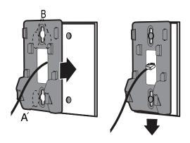
3. Align and place the telephone base on the wall mount bracket.
