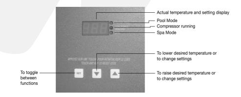
The temperature display of the electronic control panel is factory set to show pool water temperature in degrees FAHRENHEIT. See **"To select temperature in °C or °F"** section on the following page.
