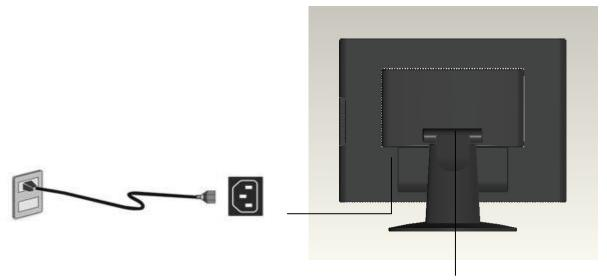
**NOTE**: For wall mount option, carefully remove back cover here.
