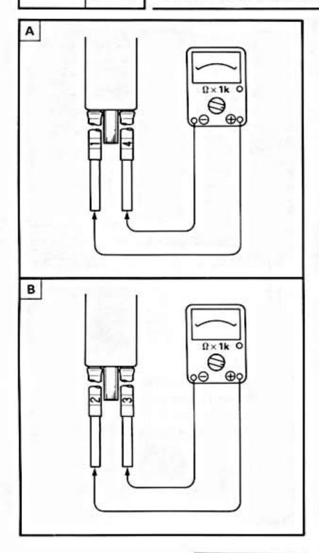
Connect Pocket Tester (YU-03112) to spark plug leads.
