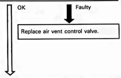
Check entire air vent control valve system for connections.
