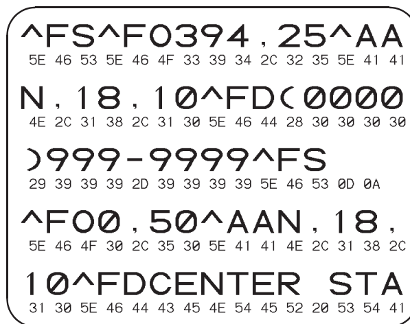
Figure 23. Communications Diagnostics Self-test
